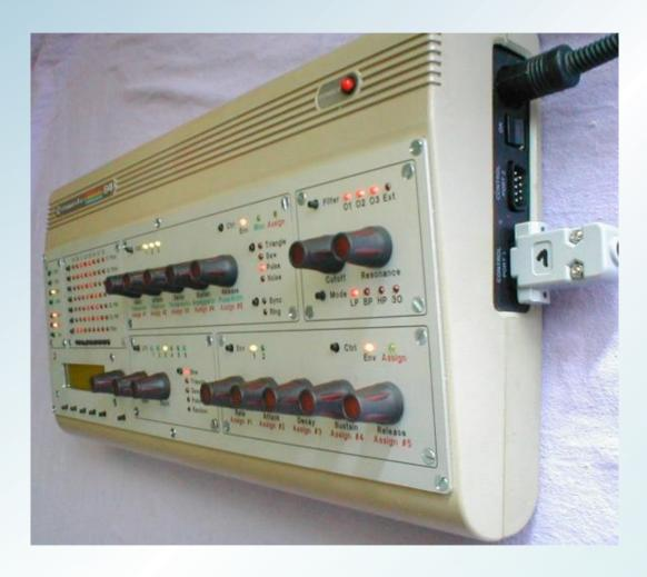
**MIDIbox SID features** more software implemented highresolution modulation sources (LFOs, EGs), independent sound engines for all 3 voices and a low-latency MIDI interface (no note drops...) - these capabilities can only be realized with a CPU that runs much faster than the 6502.
